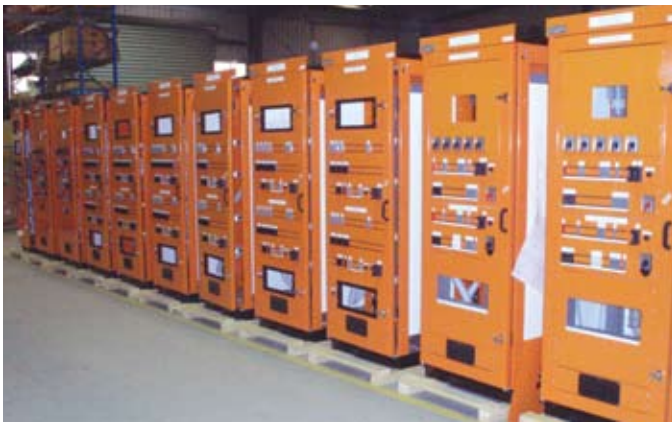
Tamco Australia's Protection and Control Panels for 33kV GIS Switchgear supplied to Integral Energy NSW
